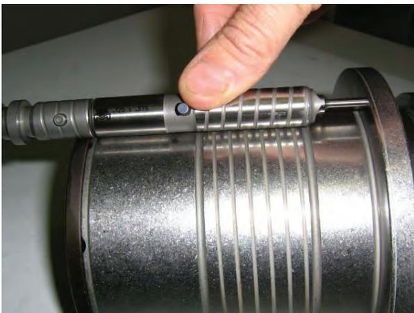
Quickly adjust the length of your punches by using the built-in length guide. Place the tip of the punch against the flange and rotate the punch driver to the guide body edge
