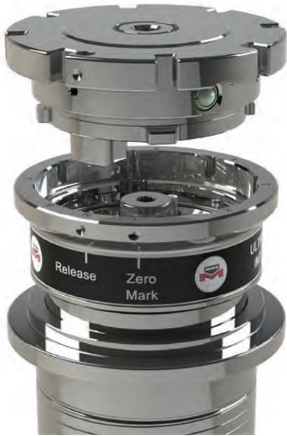
**ULTRA IMT** is designed to minimize your effort and maximize your uptime because you don't need tools to remove the striker plate, change punches, or for routine maintenance. Simply twist the striker plate to align the release dimples and remove. How easy is that!
