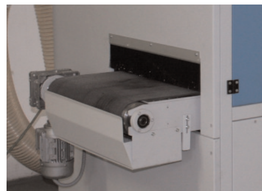
dust collection box with brush strip
