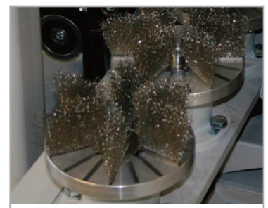
Stainless steel wire brushes for oxide removal
