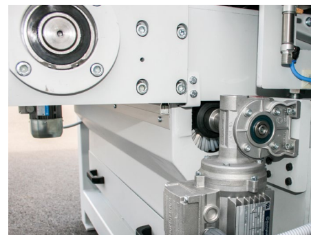
Rotating cleaning brush for feed belt (optional)
